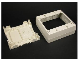
Accepts all standard two-gang NEMA faceplates and keystone jacks. Twistouts on all four sides for PN03, PN05, and PN10 Series Raceways. Has 1/2" and 3/4" concentric trade size KOs, as well as rectangular KO for wall box mounting. Designed for use with Ortronics WiJack Wireless Access Point.
