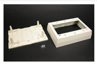
Accepts all standard 3-gang NEMA faceplates and keystone jacks. Twistouts on all four sides for PN03, PN05, and PN10 Series Raceways. Has 1/2" and 3/4" concentric trade size KOs, as well as rectangular KO for wall box mounting. Designed for use with Ortronics WiJack Wireless Access Point.
