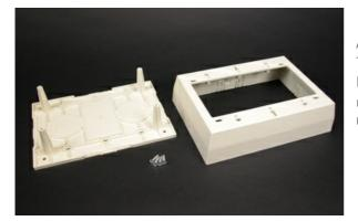
Accepts all standard 3-gang NEMA faceplates and keystone jacks. Twistouts on all four sides for PN03, PN05, and PN10 Series Raceways. Has 1/2'' and 3/4'' concentric trade size KOs, as well as rectangular KO for wall box mounting. Designed for use with Ortronics WiJack Wireless Access Point.
