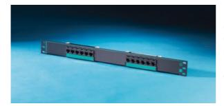
Clarity 5E 12-Port Patch Panel is component compliant to EIA/TIA Category 5e performance requirements. Standard density design provides additional space for cabling and occupies one rack unit, measuring 19'' x 1.75''. Jacks are grouped in six-port modules. Part of the Clarity 5E link and channel solution that provides significant installed performance headroom.
