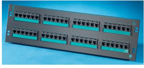
Clarity 5E 48-Port Patch Panel is component compliant to EIA/TIA Category 5e performance requirements. Standard density design provides additional space for cabling and occupies three rack units, measuring 19'' x 5.25''. Jacks are grouped in six-port modules. Part of the Clarity 5E link and channel solution that provides significant installed performance headroom.
