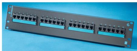
Clarity 6 24-Port Category 6 patch panel is component compliant to EIA/TIA Category 6 performance requirements. Standard density design provides additional space for cabling and occupies two rack units, measuring 19" x 3.5". Jacks are grouped in six-port modules. Part of the Clarity 6 link and channel solution that provides significant installed performance headroom.
