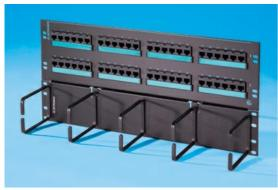
Clarity 6 48-port standard density patch panel with hinged cable management panel is component compliant to TIA/EIA Category 6 performance requirements. It occupies five rack units, and measures 19" x 8.75". Jacks are grouped in six-port modules. It is part of the Clarity 6 link and channel solution that provides significant installed performance headroom.
