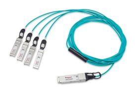
1m Siemon Q4S10F-V01.0M13 Compatible 40GBase-AOC QSFP+ to 4 x SFP+ Breakout (MMF, 850nm, LSZH) Active Optical Cable
