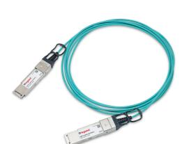
5m Cisco QSFP-H40G-AOC5M Compatible 40GBase-AOC QSFP+ to QSFP+ (MMF, 850nm, LSZH) Active Optical Cable
