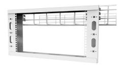
Overhead rack to support additional rack space above existing racks or cabinets. Easily installs to wire cable tray, tubular runway, or threaded rod. The racks are fully assembled and bonded as packaged. The racks are available in 2RU thru 8RU, in black or white to match any installation. Used when floor space is at a premium or for easy top of rack cable patching.
