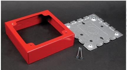
For surface mounting of alarm devices and safety signals designed to fit into 4" (102mm) square back boxes. Cover has three raceway twistouts on each side. Base has 1/2" and 1" concentric and single-gang box KOs. Available in red and ivory finishes. Accepts NEMA double-gang standard faceplates.
