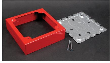
For surface mounting of alarm devices and safety signals designed to fit into 4'' (102mm) square back boxes. Cover has three raceway twistouts on each side. Base has 1/2'' and 1'' concentric and single-gang box KOs. Available in red and ivory finishes. Accepts NEMA double-gang standard faceplates.
