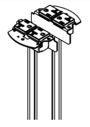
Prewired snap-in 20A receptacle can be wired as standard duplex or isolated ground. Available only in black. See installation instructions with replacement receptacle for complete installation details.
