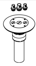
2" trade size conduit stem, complete with one 3/4" trade size conduit and two 1/2" trade size adapters and closure plugs. Finish flange/cover assembly available in painted gray (GY), black (BK), brushed plated brass (BS), and brushed aluminum (AL). NOTE: Assembled with scrub water gasket. For use on tile or carpet floors. RC9AM2TC Series Poke-Thru Devices require a 3" (76mm) diameter hole. Not designed to work with bare concrete or terrazzo. Floor covering thickness 1/8" minimum.
