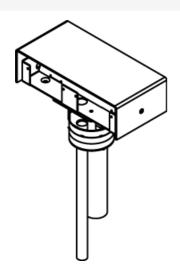
Includes insert stem with disposable plate and four-gang service head with housing, base, scrub water gasket, and barrier. Service head and insert install together to make a poke-thru assembly. Combine with faceplates (sold separately) to complete service head assembly. Shown assembled. Service head is shipped unassembled with the insert stem. NOTE: Assembled with scrub water gasket. For use on tile or carpet floors. Requires a minimum 3 1/16" (78mm) diameter hole.
