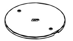
Abandonment available in black (BK). NOTE: To abandon the RC9 Series Poke-Thru Device, the internal gasket, and quad receptacle must not be removed in order to maintain UL Classification. Also the stem must remain in the hole.
