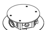
Complete with gray or black carpet flange, gray hexagonal housing, five black rubber grommets, and one 3/4" trade size threaded dropin hub. The service head includes scrub water gasket. Colors available in painted gray (GY), and black (BK). Use with the RC9FFS Insert to form a complete poke-thru assembly. NOTE: RC9AFFTC Series Poke-Thru Devices require a 3" (76mm) diameter hole. Not designed to work with bare concrete or terrazzo. Floor covering thickness 1/8" minimum.
