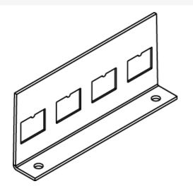
Four RJ keystone opening knockouts. Use as blank plate or for up to four RJ openings. Opening dimension is 9/16" X 3/4" [14.3mm x 19.1mm]. NOTE: For RFB4-SS Series Floor Boxes only. For use on tile, terrazzo, carpet, or wood covered floors. Additional configurations available. Please consult your local Sales Representative for more information.
