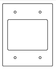
Available in two-gang sectional width. Provided with one opening to accept one Ortronics TracJack bezel and one Ortronics Series II bezel. Will accept up to six Ortronics TracJack devices or up to three dual Ortronics Series II modular inserts. Modules sold separately.
