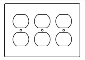
Three-gang device plate in standard (D) widths.
