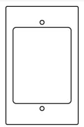
Available in standard width. Provided with bezel to accept up to three (3) dual Wiremold CM Series Open System communication modules or Pass and Seymour Activate Connectivity System inserts. Modules and inserts sold separately.
