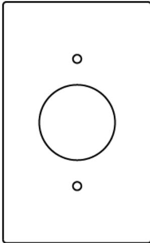
One-device plate in standard (SR) width. SR1 has an opening of 1.39" (35.31mm).
