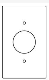
Wiremold RFB9 and RFB11 Series Single Receptacle Device Plate Part No. RFB119-SR1
