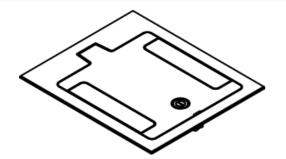
Flush with floor, cast aluminum cover assembly available in brushed aluminum (AL), black (BK), and gray (GY). Maximum load capacity 3,000 lbs. UL Listed to U.S. and Canadian safety standards to meet UL requirements under UL514A for scrub water exclusion. NOTE: Not for use on bare concrete floor applications.
