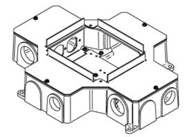
14 1/2" L x 11 7/8" W x 3 7/16" D (368mm x 302mm x 87mm). Fully adjustable with tunnel compartment and two receptacle brackets. Feed through from adjacent or opposite compartments only, (not cross compartments). Communication brackets not included. Note: Only for use in concrete floors. All boxes and activations are sold separately.
