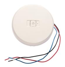
Plug load control can be easily achieved by installing the Legrand RF Receptacle into the branch wiring system and tying the low voltage RF Signal Pack into an occupancy sensor and 24Vdc power pack (PWP120277). The two are bound by a reliable wireless, RF connection. The RF Receptacle features an internal relay to switch the plug load on/off according to the sensor's command. The receptacle's feed-thru capability offers a simple and efficient means for energy savings and code compliance.
