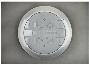
For RPSFB, RFSFB-OG, and RPNFB floor boxes. Kit comes complete with (2) prewired 20A duplex receptables, (receptables can be wired as standard receptacle, or isolated ground), flange and slide holder, adapter ring to secure into the boxes, divider (RP-DIV), Wiremold CM series open system adapters (unloaded), Ortronics Series II and TracJack adapters. Modular jacks sold seperately.
