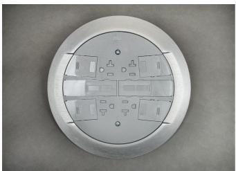
Rachet-Pro™ Series Multi-Service RC4 Style Cover Kit works with RPSFB, RFSFB-OG, and RPNFB floor boxes. Kit comes complete with (2) prewired 20A duplex receptables, (receptables can be wired as standard receptacle, or isolated ground), flange and slide holder, adapter ring to secure into the boxes, divider (RP-DIV), Wiremold CM series open system adapters (unloaded), Ortronics Series II and TracJack adapters. Modular jacks sold seperately.
