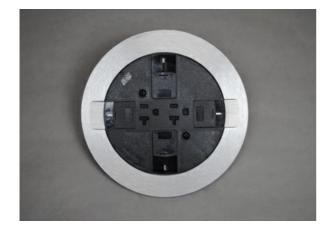
Kit comes complete with (1) prewired 20A duplex receptacle, (receptacle can be wired as a standard receptacle, or isolated ground), flange and slide holder, adapter ring to secure into the boxes, divider (RP-DIV), Wiremold CM Series open system adapters (unloaded), Ortronics Series II, and TracJack adapters. Modular jacks and A/V connectors sold separately.
