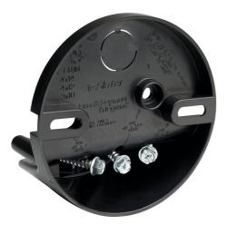
Ceiling Fan Box with Direct Mount. Suitable for Single or Double Joist.Easy installation. One #10 x 1 1/4 inch screw holds the box at rough in. Two factory-supplied #10 x 2 inch screws secure the fan or fixture through the box, directly to the joist. UL Listed for fan and fixture support.
