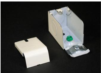
Connects 2000 Series Raceway to 1/2" trade size conduit or armored cable connectors. 1/2" trade size KOs located on end, sides, and bottom of fitting. Includes ground screw. If more capacity is required, use 2010A3.
