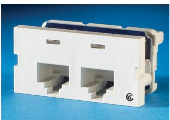
Clarity 6 Series II module two jack ports (1 unit), ETL verified to TIA Category 6 component specification. Front-loading and front removable. New universal T568A/B wiring label and tapered wiring towers simplify termination. Center tuned to Clarity 6 patch cords for optimum performance. 1800
