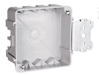
4-inch Square Box with Threaded Mounting Holes for Wood and Steel Stud Mounting. Three Auto/Clamps each end, 2 on side opposite bracket. Two #8 mounting screws factory installed.
