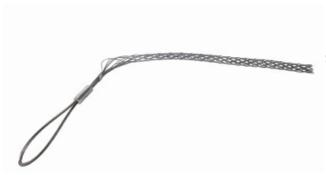
Double Weave, Standard Length, Closed Mesh, Offset Eye. Cable Diameter - 1.750-1.990-inch, Mesh Length - 19-inch, Break Strength- 11,000 lbs.
