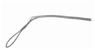
Double Weave, Standard Length, Closed Mesh, Offset Eye. Cable Diameter - 1.750-1.990-inch, Mesh Length - 19-inch, Break Strength- 11,000 lbs.
