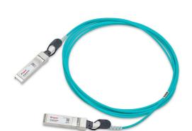
12m Cisco SFP-25G-AOC12M Compatible 25GBase-AOC SFP28 to SFP28 (MMF, 850nm, LSZH) Active Optical Cable
