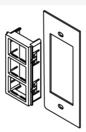
This blank plate accepts three (3) Ortronics TracJack inserts.
