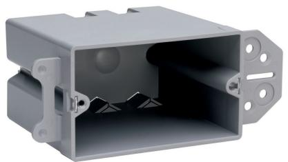
Single-Gang. Horizontal. 1/2-inch offset for wood or steel stud mount. Two stabilizer legs. 100 pack.
