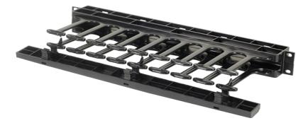
Single Sided Horizontal Managers are available in 1RU and 2RU sizes. The unique finger design protects cables from damage while the cover mounts with six hinge clips to allow the door to be opened one handed without becoming "unhinged". They are designed to mount on any 19" EIA style rack or cabinet.
