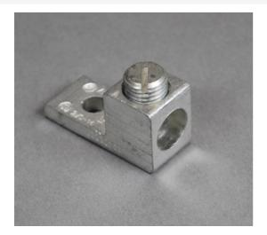
For use with SpecMate or Cablofil brand cable trays to provide ground continuity. Electroplated aluminum. Dual rated for copper and aluminum conductors, No. 2 to 14 gage cable.
