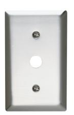
Single-Gang, Single telephone or cable outlet removable 13/32 ft ID grommet in 17/32inch fthole. Strap mounted with adjustable yoke. One #340 yoke. 302 /304 Smooth stainless steel.
