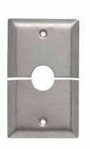
Single-Gang, Single outlet horizontal split wall plate for television or cable lead in. Box mounted, removable 5/8 ft ID grommet in 7/8-inch hole. Smooth 302/304 Stainless Steel.
