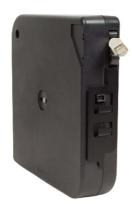
Mounts directly to the InteGreat Series A/V Table Box or to the underside of the conference room table using the TBCRHMK. Loaded with 12' (3.66m) of Cat6 cable that extends out 5' (1.52m) from the retractor. Retractor has a female input from building infrastructure, and a male connector on the output side.
