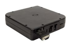
Mounts directly to the InteGreat Series A/V Table Box or to the underside of the conference room table using the TBCRHMK. Loaded with 12' (3.66m) of VGA cable that extends out 5' (1.52m) from the retractor. Retractor has a female input from building infrastructure, and a male connector on the output side.
