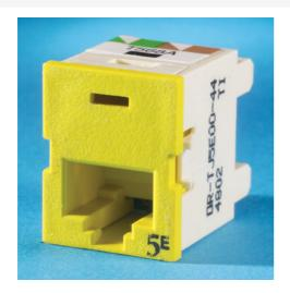
Clarity 6a, 6 & 5e TracJacks, ETL verified to TIA Category 6a, 6 & 5e component specification. Front-loading and front removable. New universal T568A/B wiring label and tapered wiring towers simplify termination. Center tuned to Clarity patch cords for optimum performance.
