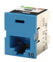
Clarity 10G TracJack, ETL tested as part of 100-meter 10 Gig channel solution. Front-loading and front removable. Universal T568A/B wiring label and tapered wiring towers simplify termination. Center tuned with synchronized reactance to Clarity 10G patch cords for optimum performance with minimized internal and alien crosstalk.
