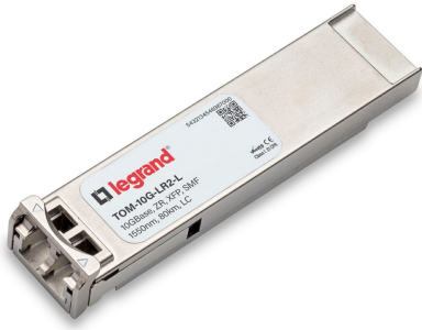
10GBase-ZR XFP Compatible Transceiver SMF, 1550nm, 80km, LC Duplex, DDM, I-Temp
