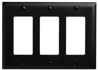
The TradeMaster® thermoplastic 3-gang decorator wall plate provides maximum durability in plastic wall plates. Self-extinguishing nylon construction makes thesewall plates virtually unbreakable. They are 3/16 of an inch higher and wider than typical plastic wall plates - not enough to be apparent to the eye, but the extra size cuts cost by reducing dry wall rework.
