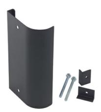
Assure the proper bend radius for cables delivered from overhead runway to equipment racks with our transition pan. Each pan clamps to runway cross members or runway stringers (TRP8-S). Truss head screws with protective covers assure cables aren't damaged. Provides 1.25 in radius.
