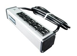
Five outlets, rugged gray aluminum housing, 15A. 6' (1.8m) 14/3 SJT black cord with NEMA5-15 plug. Length 9 1/4" (235mm). Receptacle center-to-center 1 1/4" (32mm). Snap-on, slide-off mounting.
